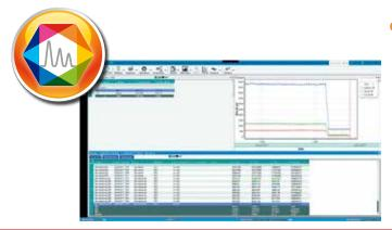
Developed by SRA, SOPRANE II performs the complete management of an analysis, from the sampling to the transmission of the results. A powerful graphical environment provides effectiveness and ease of use: it is possible to define a method and a sequence of analysis, to follow the trends for specific compounds during a TGA analysis. Soprane manages the mass spectrometer and its Agilent Masshunter software and compiles all results in a same report.
